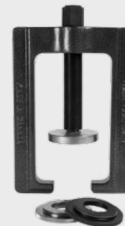
The bearing cup installer is designed for accurate installation.
