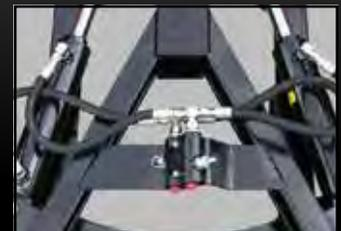
4" HD structural channel A-frame 2" kingpin with grease fitting
