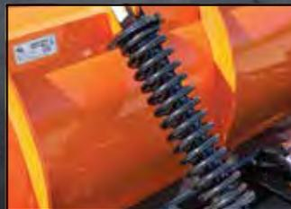
Full moldboard trip with two adjustable external compression springs
