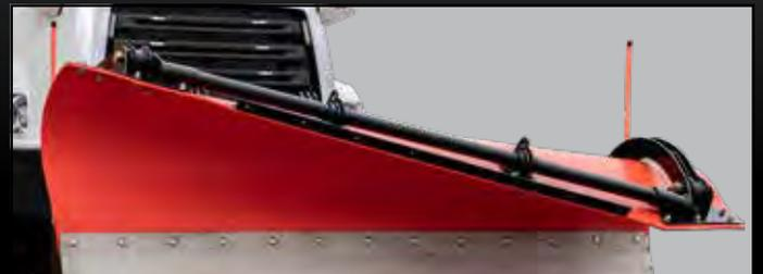
Upper moldboard cross tube provides rigidity and strength
