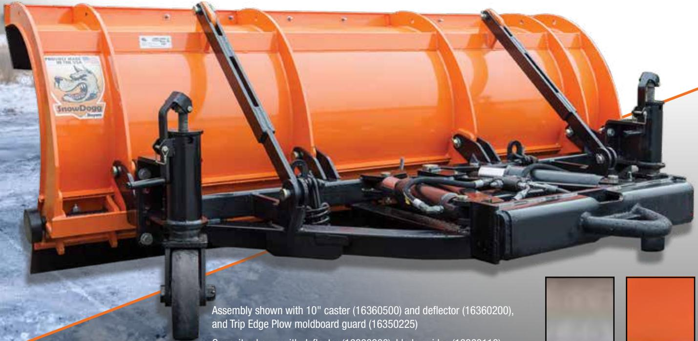
Assembly shown with 10" caster (16360500) and deflector (16360200), and Trip Edge Plow moldboard guard (16350225)
