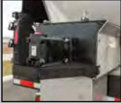
High Torque Auger Motor
