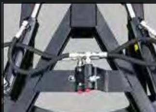
4" HD structural channel A-frame 2" kingpin with grease fitting
