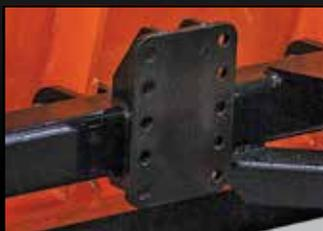
Standard mounting brackets for running gear
