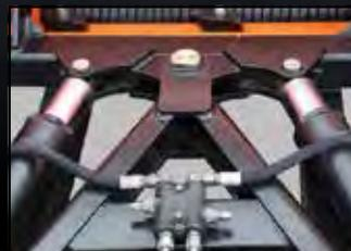
3-1/2" channel A-frame 1-1/2" king pin with grease fitting
