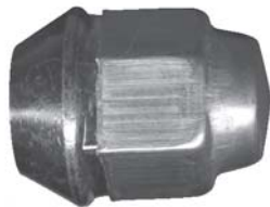
611-124 Stainless Thread Hex Size Length Seat 1/2"-20 13/16" 1-9/32" 60°
