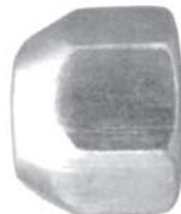
611-052 Zinc Thread Hex Size Length Seat 9/16"-18 7/8" 3/4" 60° 611-852 is a 100 pack of 611-052.
