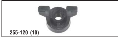
255-120 (10) Air Cleaner Wing Nut Chrysler style 1983-78. 1/4" -20
