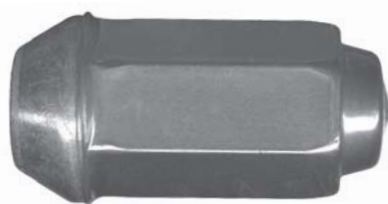
611-143 Stainless Thread Hex Size Length Seat 1/2"-20 13/16" 2-1/32" 60°
