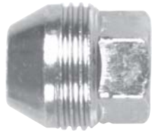
611-178 Open Nut Thread Hex Size Length Seat 1/2"-20 13/16" 1-1/8" 60°
