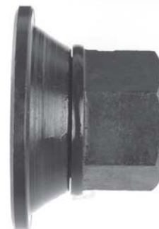
611-127 Black Oxide Thread Hex Size Length Seat 9/16"-18 7/8" 1-1/16" 1.6" dia. flange
