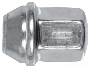
611-204 Stainless Thread Hex Size Length Seat 9/16"-18 13/16" 1-1/2" 60°
