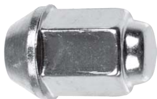
611-071 Stainless Thread Hex Size Length Seat 1/2"-20 13/16" 1-15/32" 60°
