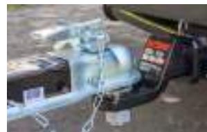
25034 securing a coupler latch
