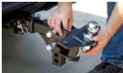
Head tilt adjustment feature simplifies setup and eliminates the need for washers
