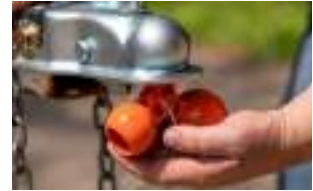
Built-in safety points allow the ball to break off when forcefully tampered with, leaving the ball in the coupler and blocking hookup
