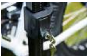
Ratcheting arms lock down onto the frames and will not loosen
