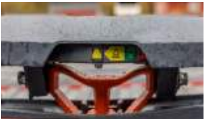
Three-position coupling indicator clearly shows coupling status
