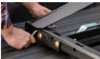
Industry-standard rails accept most 5th wheel legs and rollers
