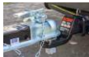
25034 securing a coupler latch
